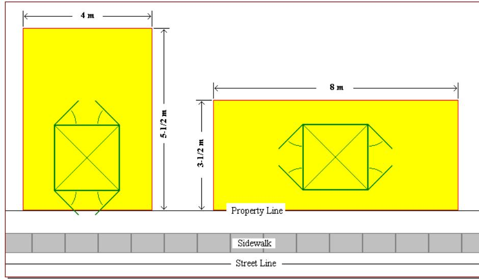
**Figure 3-4, Minimum Easement Dimensions for Padmounted Switching Enclosure**
